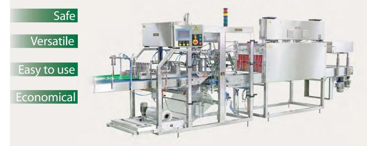
Autopack SIM CMOS is a Continuous Motion Overlap Seal bundle shrink wrapper with Inline Infeed on Multiple lanes, designed for handling all product types that can be accumulated (i.e. bottles, cans, cartons) from all industry sectors. With a maximum speed of 45 cycles/min, it is Autopack's fastest machine and among the world's most compact overlap seal machines with speed up to 135 packs/min (triple tracks).
