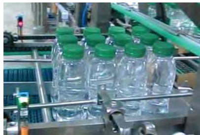
Side loading with flight bar pusher
