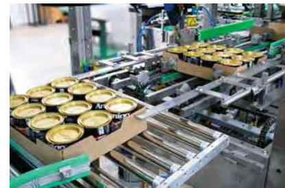
Direct connection to Shrink Wrapper
