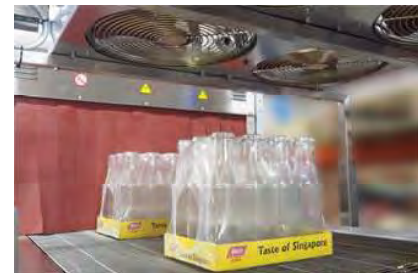
Cooling fans at outfeed
