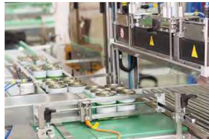
Wide infeed for preloaded trays
