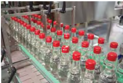
Multi lane infeed conveyor
